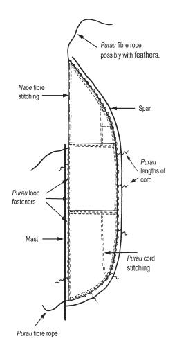
FIGURE 6. Diagram of posited sail rigging (not to scale)
